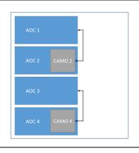
AOC 1 has a contract with CAMO 2 (in accordance with point M.A.201(ea)), AOC 3 has a contract with CAMO 4 (in accordance with point M.A.201(ea)), while CAMO 2 and CAMO 4 remain respectively integrated into AOC 2 and AOC 4 (in accordance with point M.A.201(e)(2)).
