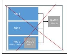
This configuration is not compliant with point  $\underline{\text{M.A.201(ea)}}$  because CAMO 1 is not contracted by AOC 3 for all the aircraft it operates.
