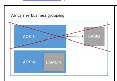
This configuration is not compliant with point M.A.201(ea) because only one AOC (i.e. AOC 1) uses the contracted CAMO.
