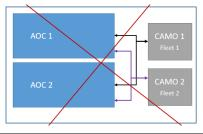
This configuration is not compliant with point M.A.201(ea) because CAMO 1 is not contracted by the AOC holders (i.e. AOC 1 and AOC 2) for all the aircraft they operate.
