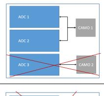
This configuration is not compliant with point M.A.201(ea) because only one AOC (i.e. AOC 3) uses the contracted CAMO (i.e. CAMO 2).
