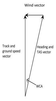
This MDR technique works for the relatively small WCAs which are typical for medium to high TAS values (the ground speed (GS) therefore can be assumed to be equal to the TAS for application of the 1:60 rule).
